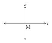
Drawing a perpendicular to a line at a point on the line.
