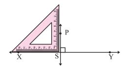
Slide the set square along the line in such a way that the other arm of its right angle touches point P. Draw a line along this side, passing through point P. Name the line PS.
